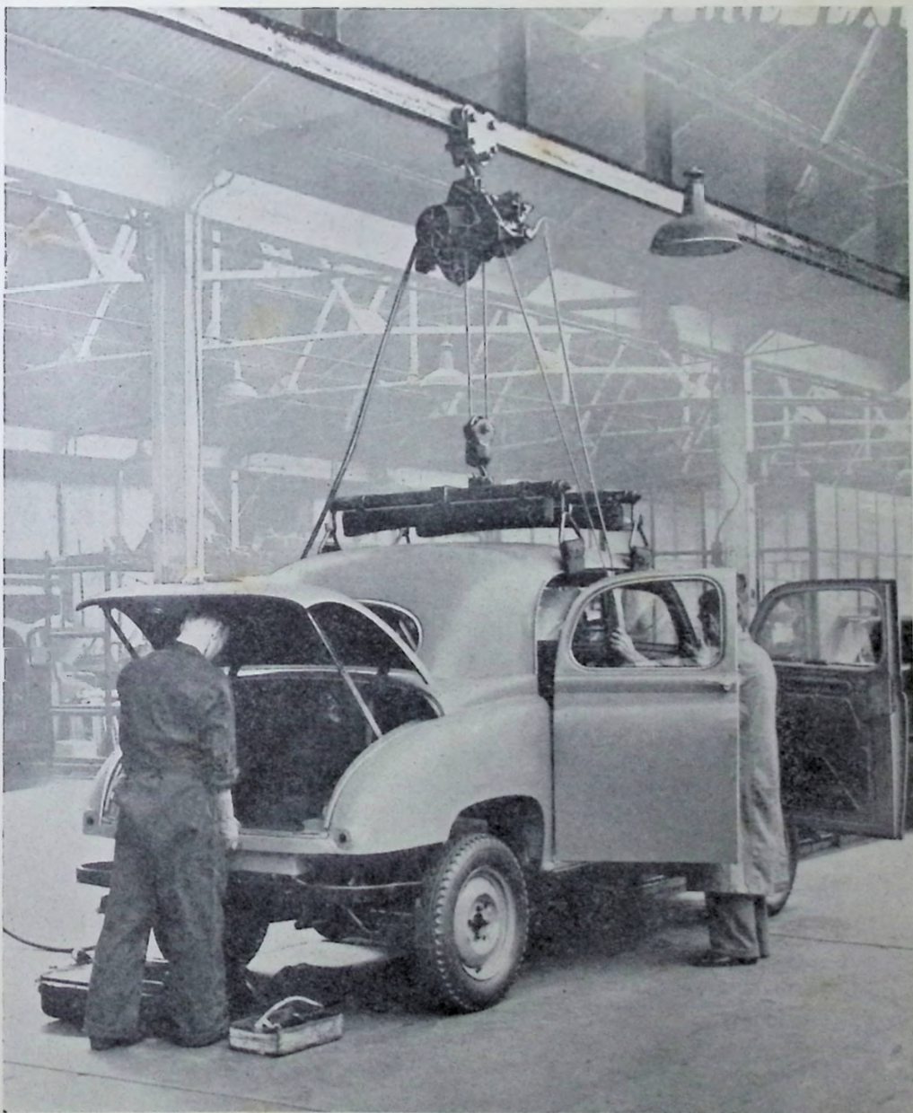
Fig. 1. Mounting the Body. Type of sling which should be used.
