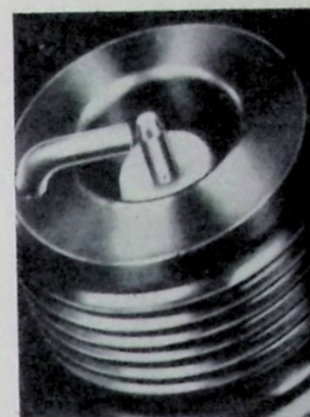
Fig. 5. New, clean, efficient plug.
