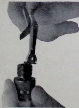
Fig. 7. Setting the Gap between the Sparking Plug Electrode.
