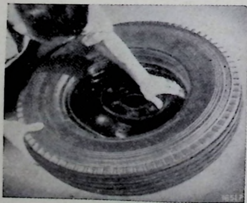
FIG. 14.—Fitting the cover. Note that the bead is pressed well into rim.
