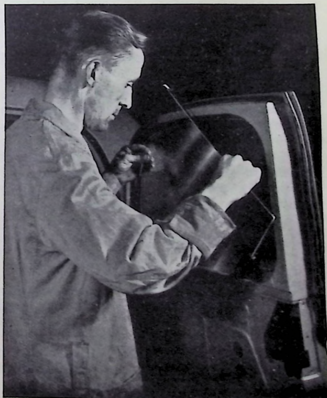
Fig. 8. Fitting Rear Door Light.
