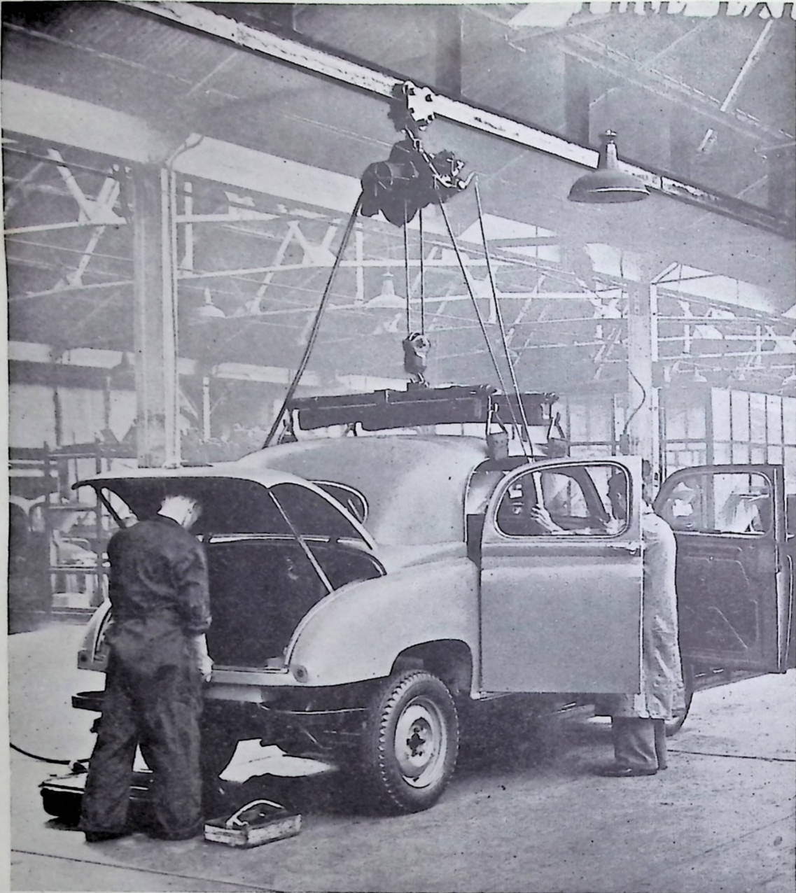
Fig. 9. Mounting the Body. Type of sling which should be used.
