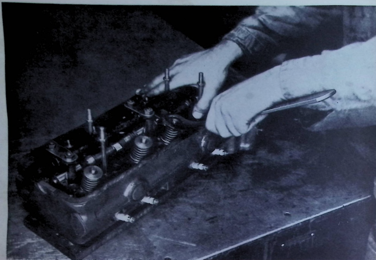
Fig. 6. Valve Extracting Tool in use.
