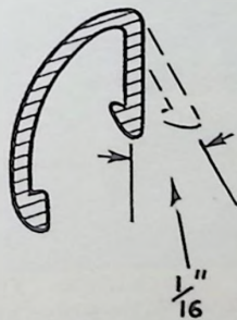
OPEN FLANGE ON OUTSIDE CHROME MOULDING AT CORNERS AS SHEWN TO ENABLE EASY START
