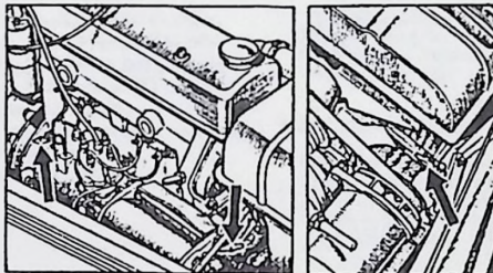
Left: Cylinder block and water pump drain taps. Right: Radiator drain tap. All on off side. System is pressurised.
